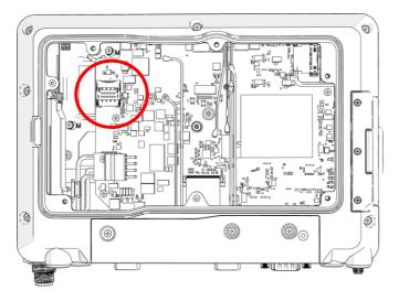
5. To release the SIM card holder, slightly lift the front edge of the cover on the card holder and slide it backwards. Open the cover.
