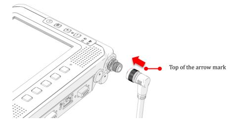
3. Twist the nut to lock the power connector to the device.
