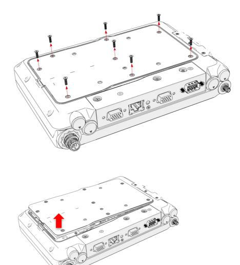
4. Once the service cover is removed, you can see the Micro SIM card slot.
