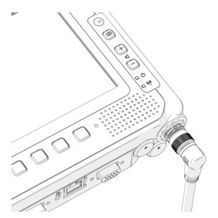
4. MT7010 will turn on automatically when the power supply is connected to the device.
