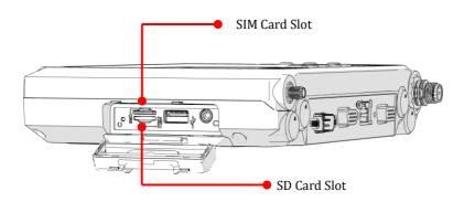
3. Insert your SIM card. Make sure the angled corner of the card is positioned correctly.
